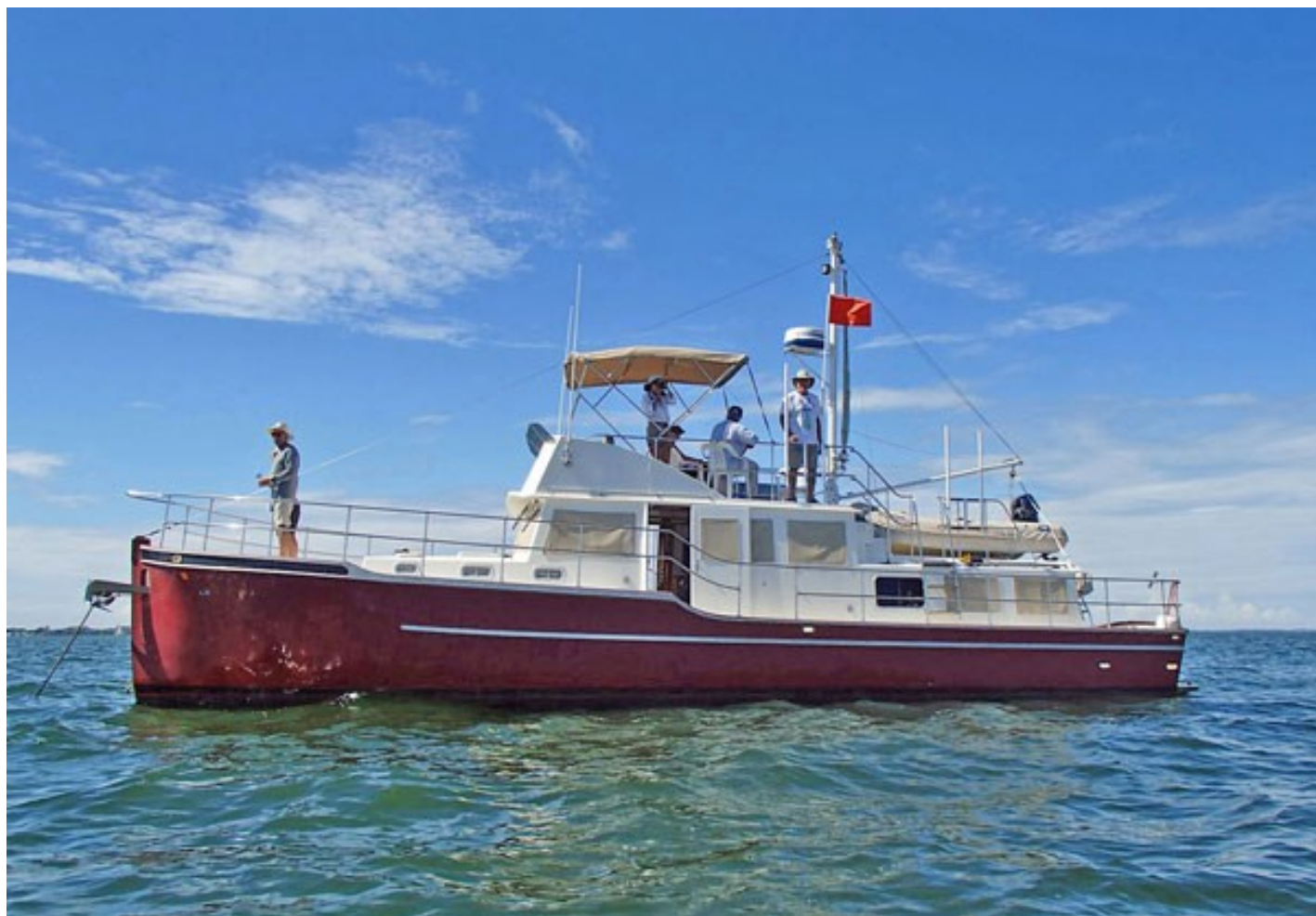
Roseate — 44-ft. beachable, tunnel-drive motorcruiser, of the Summer Kyle Class, designed by Dave Gerr
